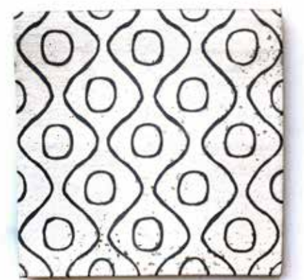
6" Pattern #6: Cast Iron (5350 Hz)
